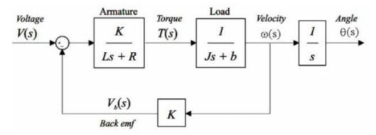
Designing a PID controller to control the position angle of the DC motor. Using Matlab codes as well as Simulink block diagram with a P-controller, assuming Kp=100, then use PID controller with Kp=1, Ki=0.8, and Kd=0.3. Comment on the changes in the output response with the P or PID controller.
