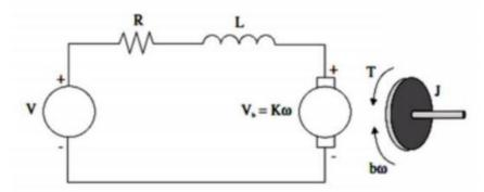
Consider the following values for the motor parameters: moment of inertia of the rotor J =0.01 kg. m2, damping friction of the mechanical system b =0.1 Nms, back electro motive force constant K =0.01 Nm/A, electric resistance R = 1  $\Omega$  ,electric inductance L = 0.5 H
